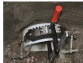
Where circumferential access is not possible FIXBLOC can be clamped to the pipe
