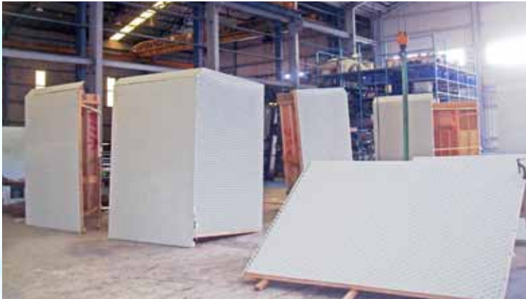
Prefabricated corners for a tank relining.
