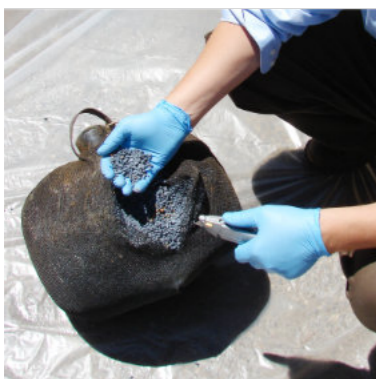
Saturated Blue media is visible through the cartridge bag.
