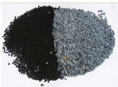
Black media on the Left is new condition. Blue media on the right is saturated media – cartridge needs replacing.
